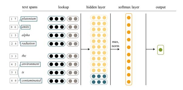
Figure 1: Layers of the Feedforward Neural Network with enriched features.
