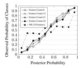
Figure 5: Reliability diagram for a Perplexed Bayes classifier with the *attenuation coefficient* optimized for good calibration a validation set, and a Naive Bayes (NB) curve for comparison.
