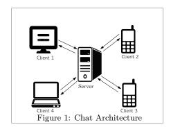
Figure 1 shows the system architecture of *TransChat.* Our system consists of a highly scalable chat server ejabberd<sup>3</sup> based on *Extensible Messaging and Presence Proto* $col(XMPP)^4$  protocol.
