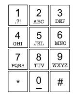
Figure 1: Standard 12-button keypad layout (ISO 9995-8).
