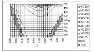
Figure 5. Kurtosis in the power spectrum of the synthetic vowels plotted against the formant values. The analyzed area is marked with boundaries.
