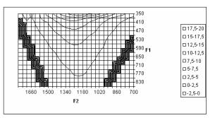
Figure 4. Skewness in the power spectrum of the synthetic vowels plotted against the formant values. The analyzed area is marked with boundaries.
