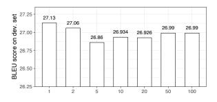
Figure 2: The effect of using different Ks when approximating distillation loss with K-most probable actions in the machine translation experiments.
