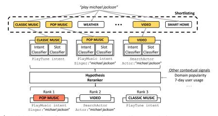
Figure 1: A high-level flow of our two-step shortlisting-reranking approach given an utterance to an IPDA.
