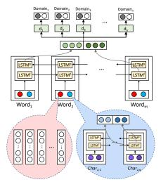
Figure 2: The architecture of our neural shortlisting model that uses character and word-level information of a given utterance.
