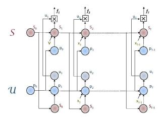
Figure 2: The sentence-encoding subnet S and the unbinding subnet U are inter-connected LSTMs; v encodes the visual input while the  $x_t$  encode the words of the output caption.
