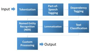
Figure 5: Processing steps in spaCy pipeline, it starts by giving the input. The outcome will include linguistic annotations after all the processing steps.
