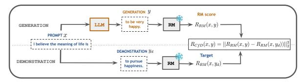
Figure 1: The RCfD objective is the L2-distance between the reward from the LM and the reward from the demonstration. Given a prompt x, a demonstration  $y_d$ , and the LLM continuation y, the RM computes the demonstration reward  $R_{RM}(x,y_d)$ , and the LM reward  $R_{RM}(x,y)$ . Instead of maximizing R(x,y) as in standard RL, we here aim at maximizing the RCfD objective defined as  $R_{RCfD}(x,y) = -||R_{RM}(x,y) - R_{RM}(x,y_d)||_2^2$ .
