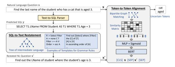
Figure 3: Illustration of Error Locator with a real case from IRNet on the Spider dataset. The NL question x is parsed to SQL y, and then converted to restated NL question x' via SQL-to-text restatement. Then, a token-to-token alignment similarity matrix between x and x' is computed to detect uncertain tokens (i.e., cat and aged).
