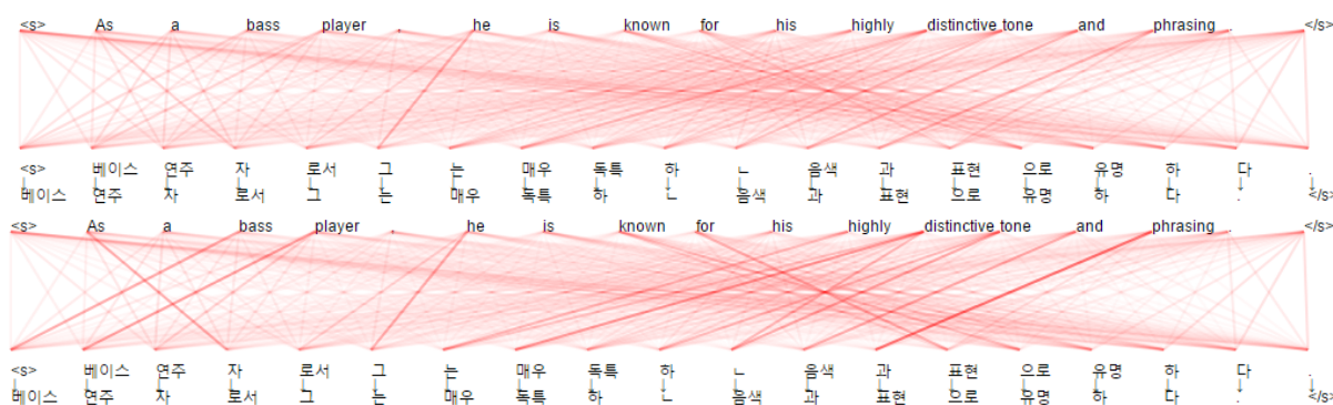
Figure 10: Two attention graphs of en-ko NMT. The first one shows attention weights from NMT. The second one shows attention weights adjusted to maximize target sentence. It reveals clearer and more interpretable relation than original attention.
