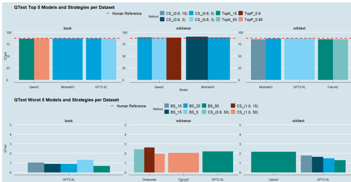
Figure 2: Top five and bottom five decoding strategies, based on QText averages for each dataset. The highest-ranking strategies generally strike a balance between coherence and diversity, while the lowest-ranking strategies tend to overemphasize one at the expense of the other—such as beam search, which favors coherence, or contrastive search with \alpha = 1.0 and k = 50 , which prioritizes diversity.
