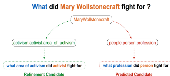
Figure 1: Sketch of our approach. Elements in solid round rectangles are KB relation labels. Relation on the left is correct, but the base QA system predicts the one on the right. Dotted rectangles represent revised questions with relation labels plugged in. The left revised question looks semantically closer to the original question and itself is more consistent. Hence, it shall be ranked higher than the right one.
