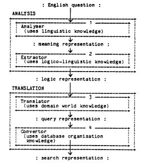
Each process in the diagram above operates on the output of the previous one. Processes 1 and 2 constitute the analysis phase, and processes 3 and 4 - the translation phase. Such a system has essentially been constructed, and is under active test; a detailed account of its components and
