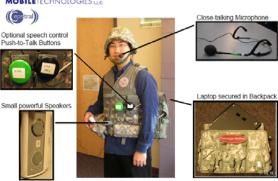
Figure 2: Hardware components
