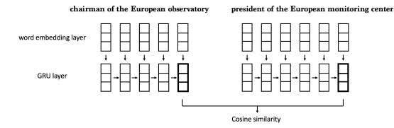
Figure 1: PGRU encodes phrase pairs with two GRUs which share the same parameters regardless of phrase lengths. Similarity is calculated by multiplying the two last hidden states with dot product.
