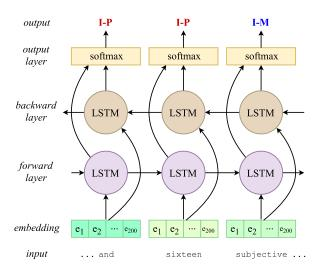
Figure 7: The NN stack using Bi-LSTM. An embedding at each word step is fed into forward and backward LSTM layers, which are fully connected to a softmax-activated output layer. (For the unidirectional LSTM, the backward layer is omitted.)
