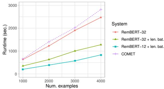
Figure 5: Runtime varying number of examples. We ran each experiment 3 times and averaged the results, using a Google Cloud VM with 4 Intel Haswell vCPUS, 15GB main memory, and an nVidia Tesla T4 GPU. COMET uses the model wmt-large-da-estimator-1719.
