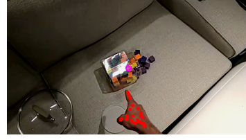
Figure S1: Example of multimodal eye gaze and hand gesture overlay for the image input Vision-Language Model (VLM). MICA uses visual prompting to indicate gaze and gesture locations to the VLM. The user’s gaze is represented by the purple circle, while hand gestures are highlighted in red.
