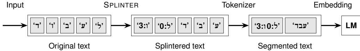
Figure 1: Overview of a Hebrew language model pipeline using the example ‘to work’: standard flow vs. incorporating SPLINTER. This figure is a real example for the differences in tokenization using a BPE tokenizer with a vocab size of 2000. Gray boxes are ordered from right to left.
