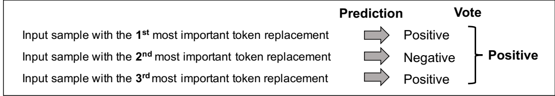
Figure 2: Step 4: The model makes a prediction after each replacement, and assigns each replacement a vote based on its prediction. The model’s final prediction is the prediction with the majority of the votes.
