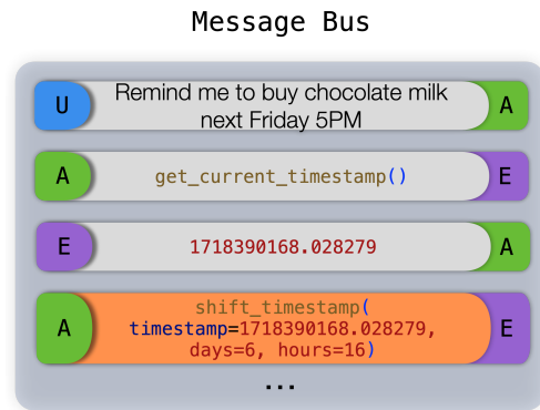
Figure 14: Example trajectories where GPT-4 incorrectly inferred relative time. Instead of deducing next Friday 5PM by inspecting current day and weekday, GPT-4 randomly shifted current time stamp by 6 days and 16 hours.
