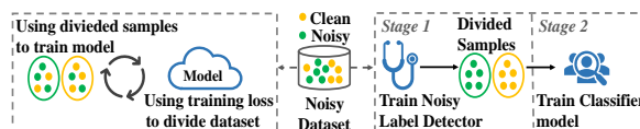
Figure 1: A comparison between other sample selection methods (left) and our method (right) for LNL tasks. Our method decouples sample selection (stage 1) from model training (stage 2) by training a noisy label detector and classifier model separately.
