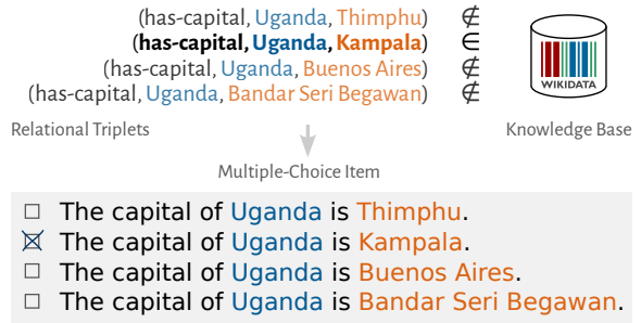
Figure 2: In BEAR, one statement per answer option is passed to the LM (here using the template: “The capital of [X] is [Y].” and the subject “Uganda”). The assigned sentence-level likelihoods are then used to rank the answer options (figure from Ploner et al., 2024).
