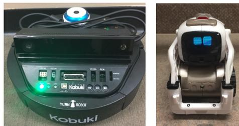
Figure 1: The two physical robots in our study: KOBUKI with a mounted MS Kinect and COZMO.
