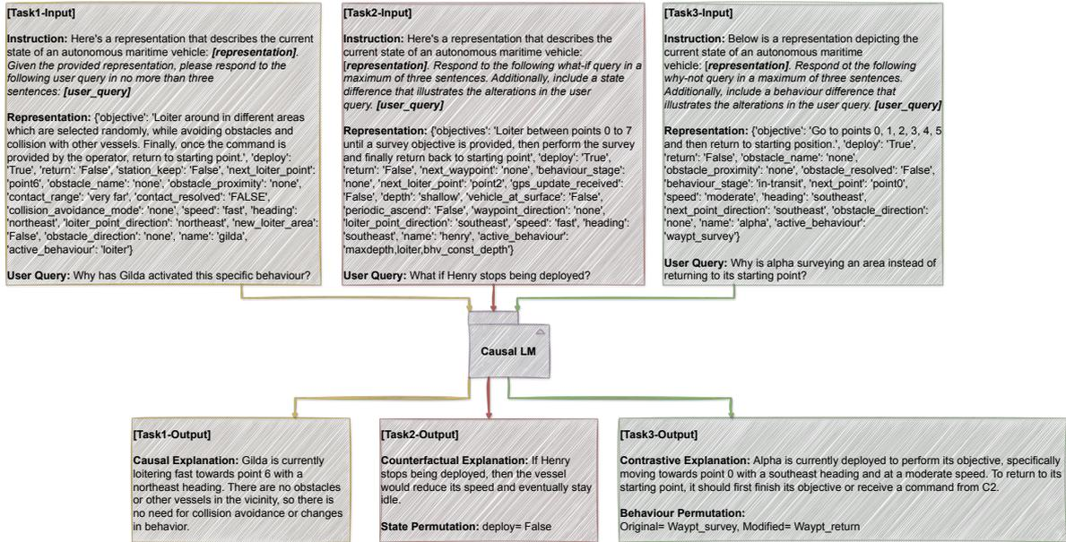
Figure 3: The defined fine-tuning tasks involve a causal language model that retrieves an instruction, a vehicle state representation, and a user query. The model then outputs an explanation, and for counterfactual and contrastive explanations, it additionally provides a permutation.
