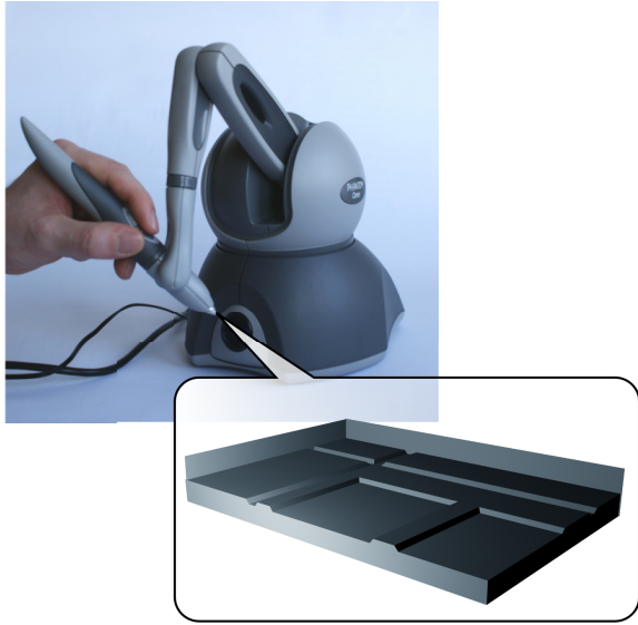
Figure 1: The Sensable Omni Haptic Device and a Visualization of a Virtual Tactile Map.
