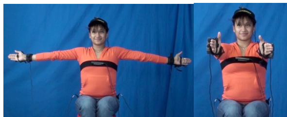
Fig. 5. Arm movements the signer was asked to perform to facilitate calibration of the collected motion capture data.
