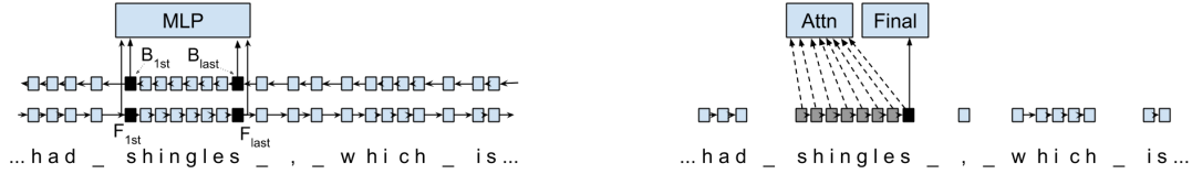
(a) Sentence-based Character Model. The representation for the token shingles is the concatenation of the four shaded boxes. Note the surrounding sentence context affects the representation.
