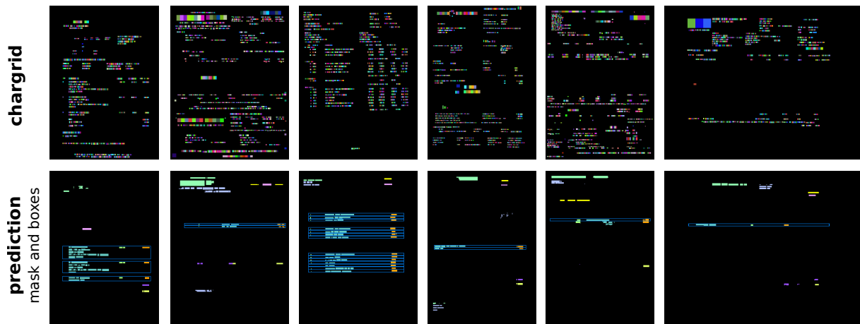
Figure 5: Sample invoices and their corresponding network predictions: the top row shows the chargrid input, the bottom row shows the predicted segmentation mask with overlaid bounding box predictions. Our model is able to handle a large diversity of layouts. The encoding of the characters on the chargrid has been scrambled to preserve privacy.
