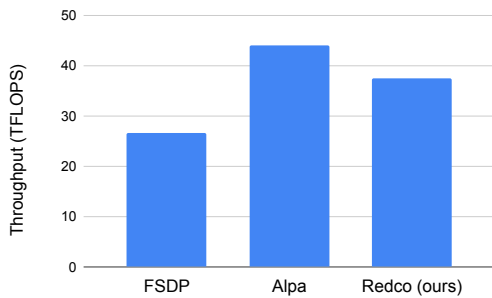
Figure 3: The comparison of throughput in the running of GPT-J-6B on a 4 \times A100 server. Redco’s performance surpasses that of FSDP and is close to that of Alpha, the tool with state-of-the-art model parallel efficiency but intricate engineering.
