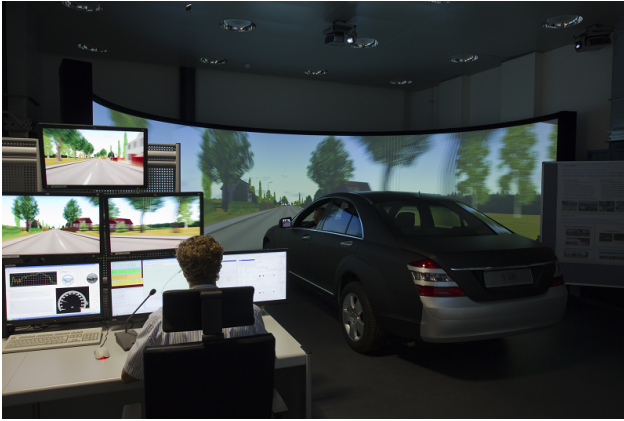
Figure 1: Driving simulator with operator desk (Schmidt et al., 2020)
