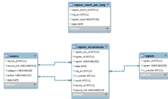
Figure 2. The database has a table for the source URIs, n-grams, n-gram counts for each language, and the n-gram occurrences which includes the URI the word was mentioned, the date the article was published, and how many times the word was mentioned in that article.
