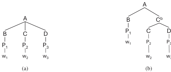
Figure 1 Example of a constituent tree (a) and a valid right binarization of it (b).
