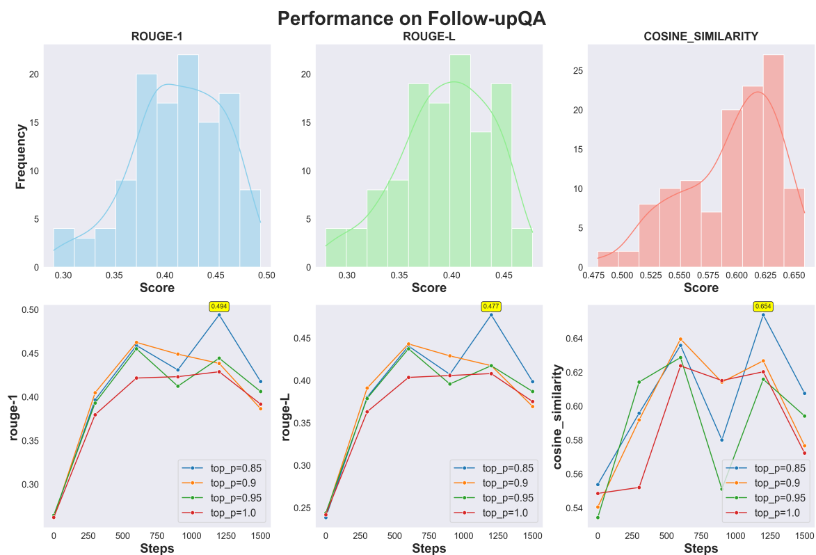
Figure 3: Benchmark Mistral-7B for Follow-upQA. First row: distribution plots for ROUGE-1, ROUGE-L, and cosine similarity across hyper-parameters. Second row: Mistral-7B performance at different training checkpoints.
