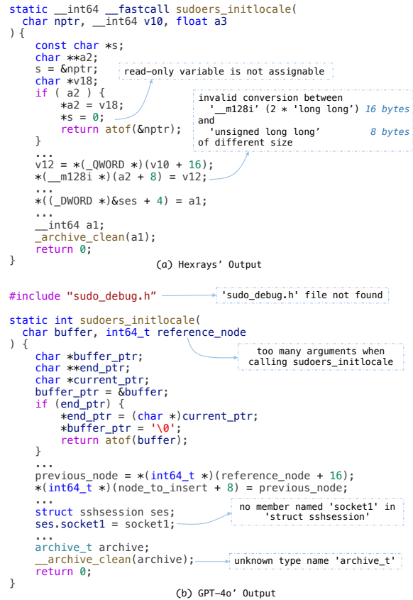
Figure 4: Output of Hex-Rays and GPT-4o. The error reports highlight where one decompiler fails and the other succeeds, demonstrating their pros and cons.
