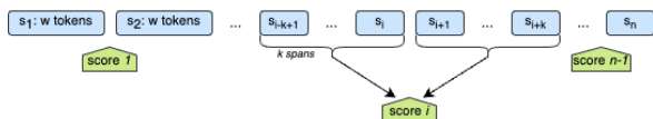
Figure 1: Segmentation in spans of w tokens and computation of the lexical scores in the TextTiling algorithm.
