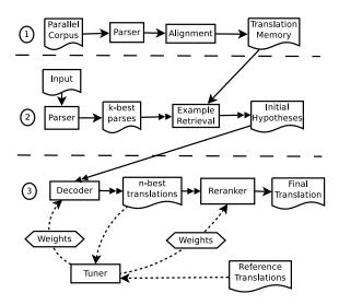
Figure 2: The translation pipeline can be roughly divided in 3 steps. Step 1 is the creation of the example database, trained from a parallel corpus. Step 2 is the k-best parsing of an input sentence and the generation of k sets of initial hypotheses. Step 3 consists in decoding and reranking. The tuning of the weights for decoding and reranking is done by a modified version of step 3. The double arrows indicate the parallel processing of each of the k parse of the input sentence.
