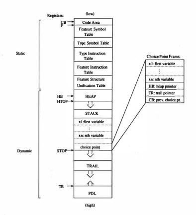
Figure 1: Abstract Machine Memory Layout and Registers
