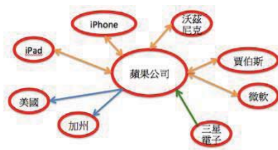
Figure 6. A link graph. Blue edges denote outlinks, green edges denote inlinks, orange edges denote both inlinks and outlinks.
