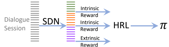
Figure 1: The workflow for HRL with subgoal discovery. In addition to the extrinsic reward at the end of the dialogue session, HRL also uses intrinsic rewards induced by the subgoals (or the ends of dialogue segments). Section 3.2 details the reward design for HRL.
