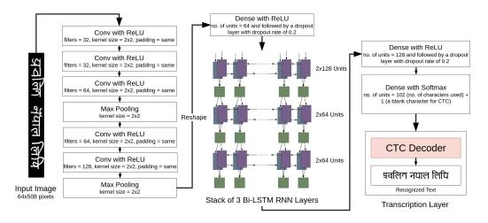
Figure 8: CRNN CTC based Nepal script text recognizer model architecture.
