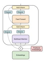
Figure 1: Transformer's attention block diagram with Residual Dropout.
