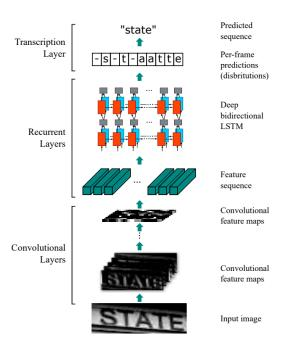
Figure 2: CRNN CTC Architecture integrating the key features of CNN, RNN, and CTC (Shi et al., 2016).
