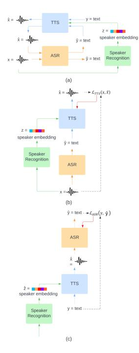
Figure 1: (a) Overview of a machine speech chain architecture with speaker recognition. Unrolled process of unsupervised training: (b) from ASR to TTS and (c) from TTS to ASR (Tjandra et al., 2020)
