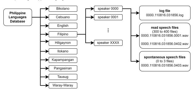
Figure 5: A diagram of the structure of the Philippine Languages Database. Collected recordings are grouped according to language and speaker, with each speaker corresponding to one folder. For each speaker, which in this example is speaker 0000, the corresponding folder contains the speech recordings stored in WAV format and the log file which contains the transcripts.
