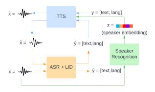
Figure 2: Overview of a multilingual machine speech chain architecture with speaker recognition (Nakayama et al., 2019)
