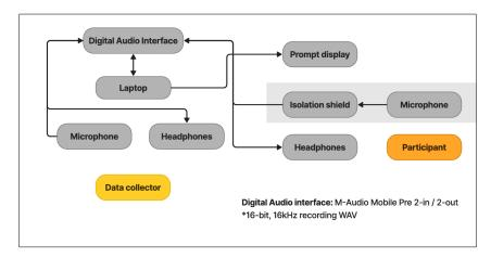
Figure 2: Diagram of the recording setup during fieldwork.
