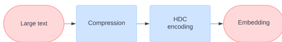
Figure 1: Workflow of the compression HDC model, illustrating the processing of a large text using text compression and HDC encoding (blue), to produce a final embedding.
