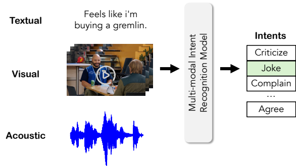
Figure 1: An example of multi-modal intent recognition (MIR), where intent cannot be easily inferred from text alone. By combining a man’s smirking expression with an exaggerated tone, it can be classified as ‘Joke’.
