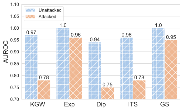
Figure 5: Comparison of the robustness of decoding-based watermark on Completion task. Blue histograms indicate unattacked conditions and red histograms show attacked scenarios. The AUROC is calculated for 40 detection tokens, with GumbelSoft set at a 0.3 temperature. Exp , Dip , and GS refer to Exponential, Dipmark, and GumbelSoft, respectively. GumbelSoft and Exponential show higher robustness when facing the T5-span attack.
