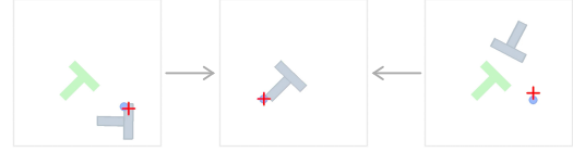
Figure 10: Astra in Push-T. The gray T is the object, and the green T is its target position. The model controls the blue dot to push the T-shaped object towards the target position. The red cross is the cursor. The images on the left and right are two different initial states, and the middle image is the final state where the object perfectly overlaps with the target position.
