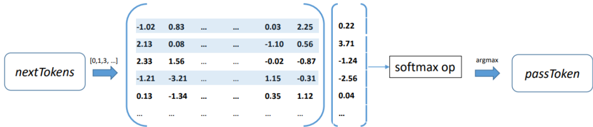
Figure 3: Integrating grammatical continuations into a log-linear model at one prediction step; rows selected by nextTokens are shaded in blue.
