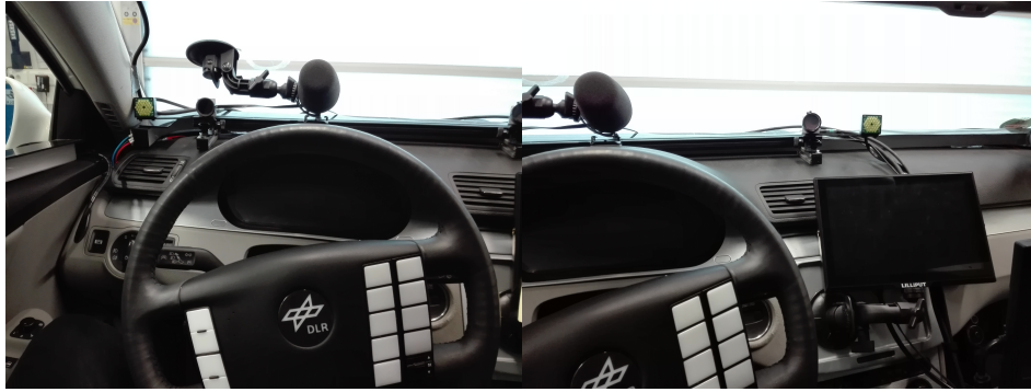
Figure 2: Setup of the microphone and SEP camera system (Smart Eye AB, Gothenburg, Sweden, www.smarteye.se ) on the dashboard of the FASCar research vehicle.
