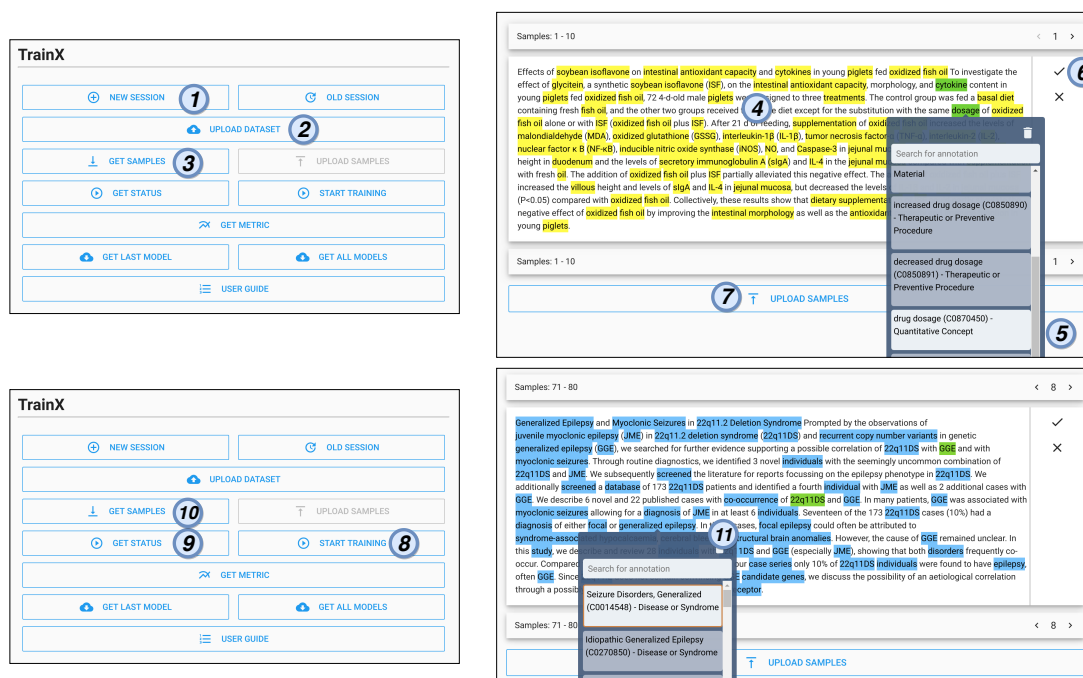
Figure 1: Usage of the TrainX system to train and evaluate the entity linker on a mixture of given GOLD and added USER labels. The screenshots show the menu, where a user requests samples or starts the training and the sample view where she can edit annotations.
