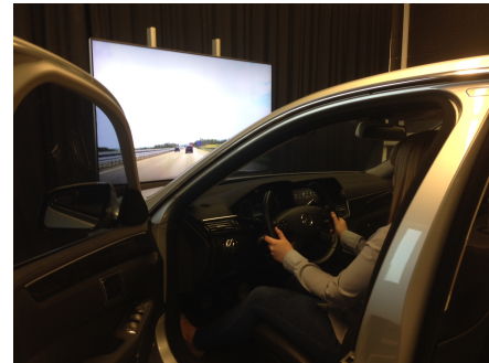
Figure 3: Driving Simulation Setup.
