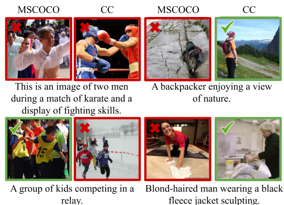
Figure 3: Comparing models trained with the MSCOCO and CC datasets. We provide the top-1 ranked retrieved image given an input query sentence on the Flickr val dataset. Correctly retrieved images are framed in green and the incorrect ones in red.
